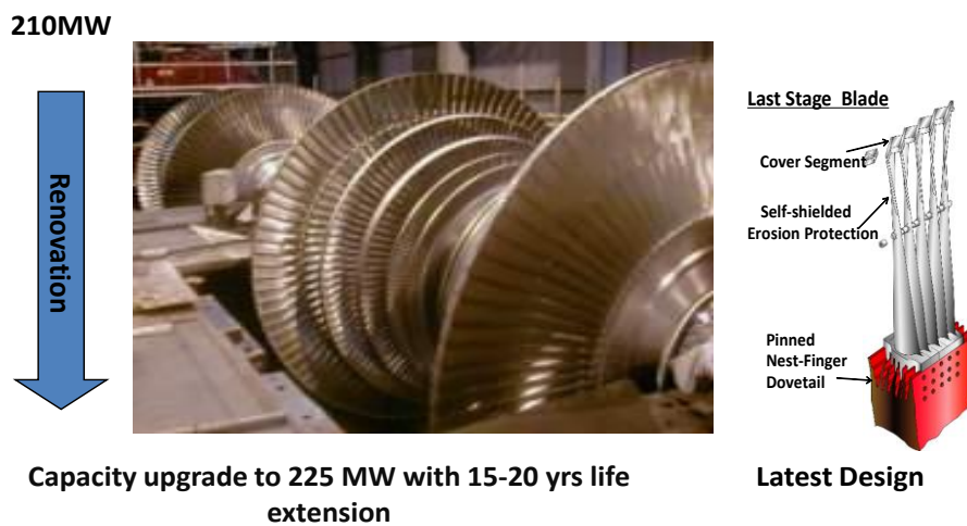
Figure 67. Turbine Restoration (Case 2) 47
