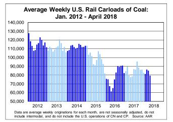
In 2016, the average length of haul for rail coal movements was 856 miles. Coal movements exceeding 1,500 miles are not uncommon. The vast majority of coal moves in gondolas and open-top hoppers.
