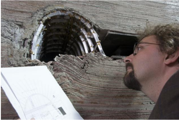
Physical modelling of ground stresses around a roadway in an underground coal mine
