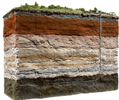
Directional drilling is used to extract coal mine methane prior to coal mining
