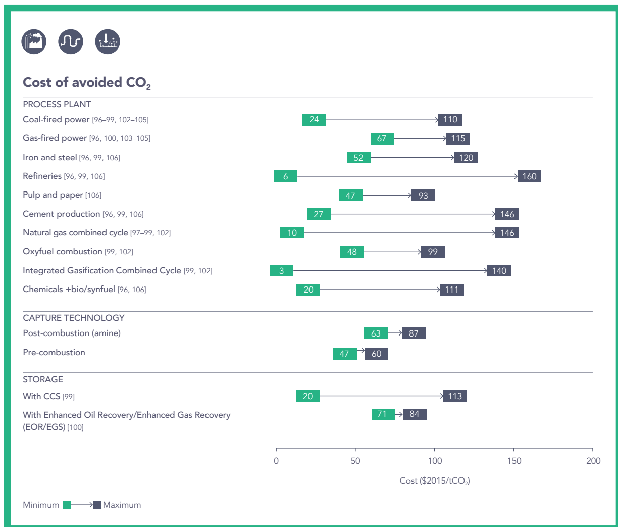
FIGURE 14 Cost of avoided CO 2 for different process plants, capture technologies and storage solutions.
