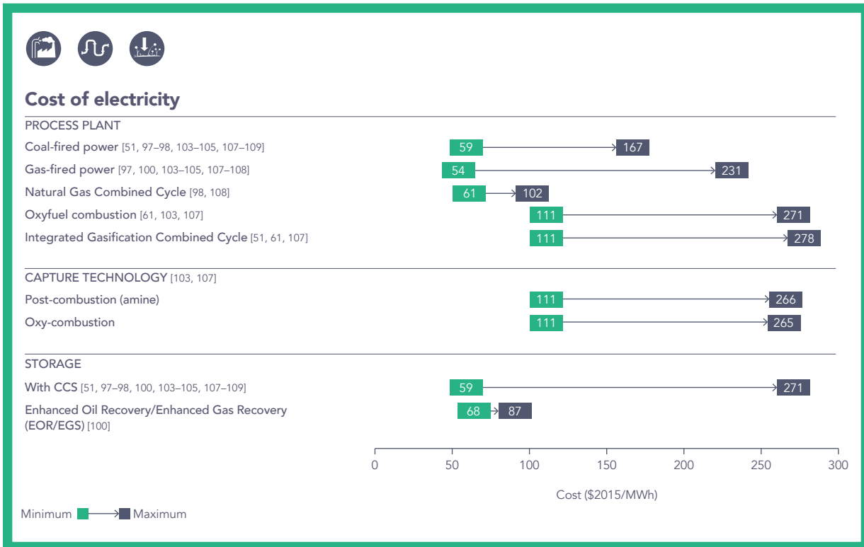
FIGURE 15 Cost of electricity for different process plants, capture technologies and storage solutions.
